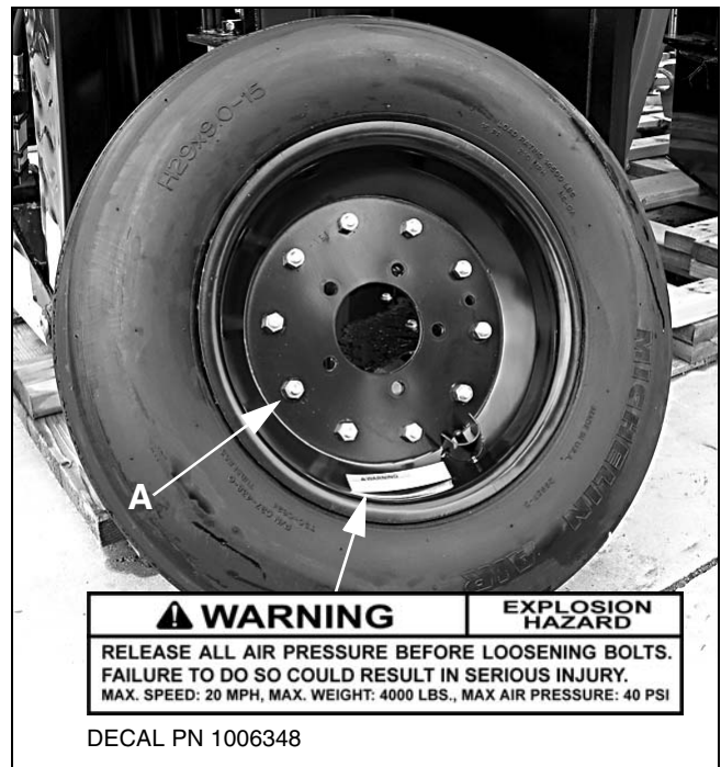
Figure 16. Split Rim Tire Servicing
